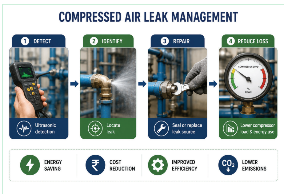
Figure 7 Compressed Air Leak Detection
